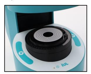
Push the Run button on the bottom right: . The instrument will proceed to perform several image captures, and finally, an image of the calibration disk will appear on the Image Panel.
