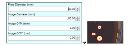
**Plate Diameter:** This corresponds to the blue circle on the image, and the user should adjust its diameter so that the blue circle perimeter matches the inner edge of the plate cylindrical wall. The application assumes that, in a spread distribution, the *Inoculated Volume* has been uniformly spread up to the limit defined by the blue circle.
